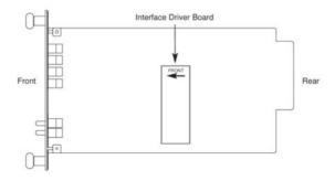
Figure 7. Driver Board mounted on Model 3088RC
